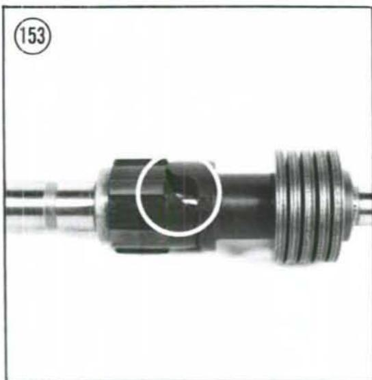
damage may be removed with an oilstone, but if damage is severe, the sprocket must be replaced. Also check the condition of the Hy-Vo chain as it may be damaged also; replace if necessary.
