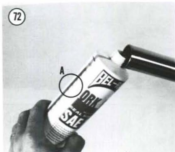
*NOTE: In order to measure the correct amount of fluid, use a plastic baby bottle. These have measurements in fluid ounces (oz.) and cubic centimeters (cc) on the side (Figure 73). Many fork oil containers have a semi-transparent strip on the side of the bottle (A, Figure 72) to aid in the measuring.*
