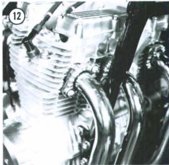
28. Have an assistant help you remove the engine from the frame through the right-hand side.
