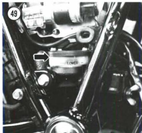
3. Reinstall the washer, diaphragm, and cap; make sure that the cap is screwed on tightly.
