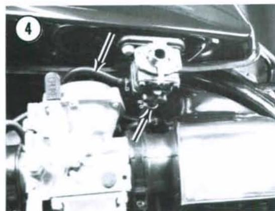
7. Loosen the 4 clamping screws on the front rubber intake tubes (A, **Figure 6**) and slide the clamps away from the carburetors.
