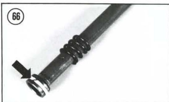
4. Inspect the oil seals for scoring and nicks and loss of resiliency. Replace if its condition is questionable.
