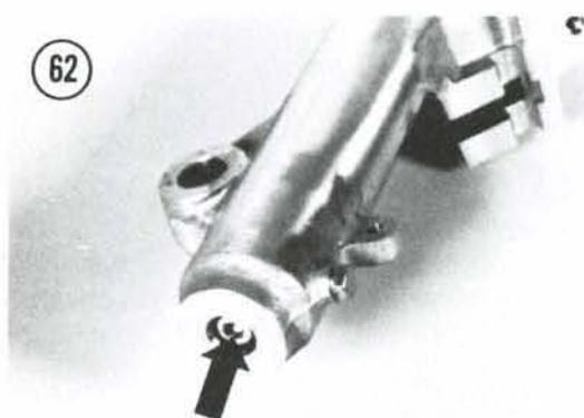
7. Clamp the slider in a vise with soft jaws.
