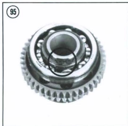
remove the bearing from the right-hand side. To remove the left-hand bearing, slide off the oil seal (B, **Figure 94**) and the bearing.
