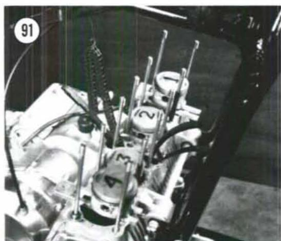
5. Remove the circlips from the wrist pin bores (Figure 94). Wrap a clean shop cloth under the piston so that the clips will not fall into the crankcase.
