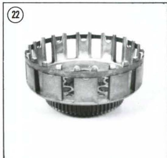
and clutch boss assembly (**Figure 23**) for cracks or galling in the grooves where the clutch friction disc tabs slide. They must be smooth for chatter-free clutch operation.
