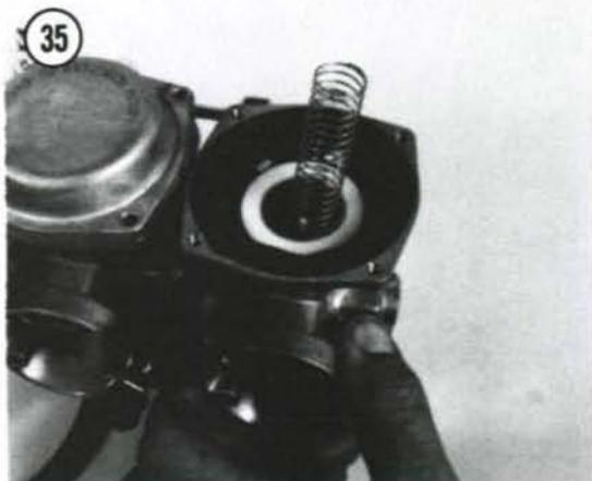
1. Remove the carburetors as described under *Carburetor Removal/Installation* in this chapter.
