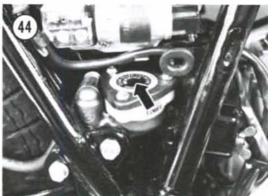
5. Continue to pump the lever or pedal and fill the reservoir until the fluid emerging from the hose is completely free of bubbles.
